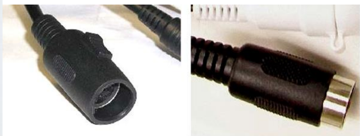
Cupped connector Good connector
